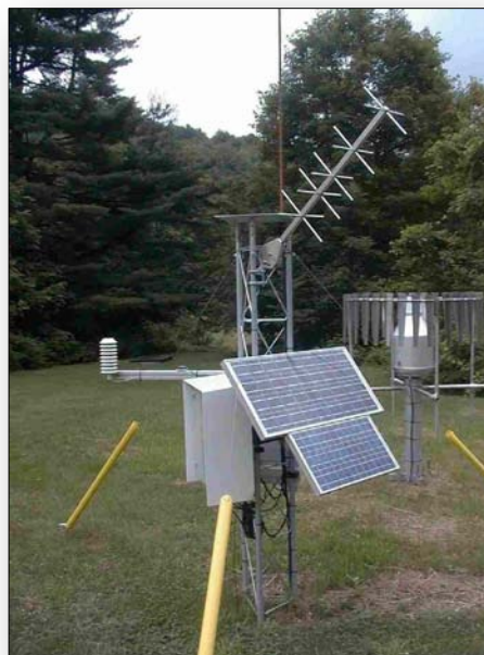
Figure 7. Cooperative NOAA Real-Environmental Real-Time Observation Network (NERON) station located at USACE's Union Village Dam in Thetford, VT. (Photo courtesy USACE New England District).
